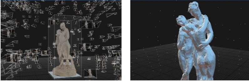
Figure 1: Close-Range Photogrammetry principle.
